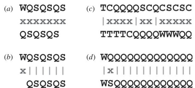
Figure 2. Examples of NW comparisons. The NW difference is calculated by counting the minimum number of pointwise differences between the two strings. (a) Two unaligned strings with an NW difference of 7. The NW algorithm aligns the strings as in (b) to minimize the NW difference. (c) Two hyrax bouts which are highly different, NW difference = 9, and (d) two bouts which are very similar, NW difference = 1. Letters indicate the different syllable types: W, wail; C, chuck; S, snort; Q, squeak; T, tweet.
